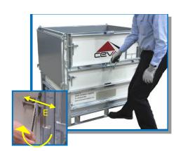
5. For final panel, again pull up using handle and secure with locking bolts (E)
